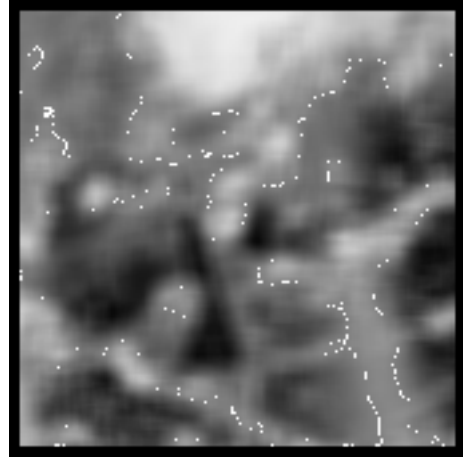
new raster after averaging pixels within 4x4 pixels of each other
